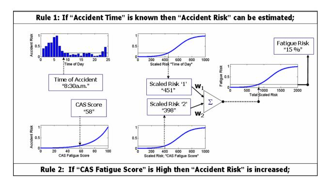
Figure 2. Rule based fuzzy mapping of normalized risk, combined into a total risk estimate, and mapped to an overall fatigue probability (for a two rule case).
