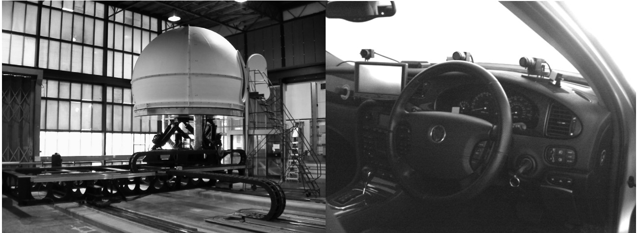
Figure 1. Exterior view and vehicle cab of the University of Leeds Driving Simulator
