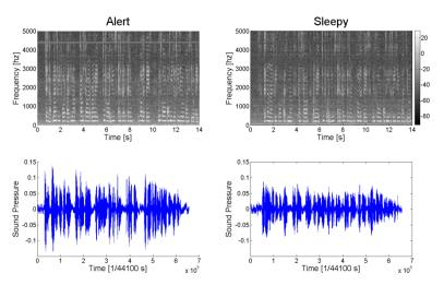
Figure 3. Spectrogram and waveform of alert vs. fatigue speech. High power spectral densities (PSD) are coded white, low PSD are coloured grey within the spectrogram.
