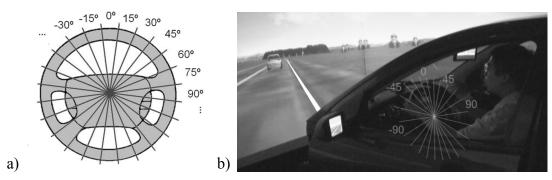
Figure 3. a) Steering wheel bins b) Bins overlaid with video
