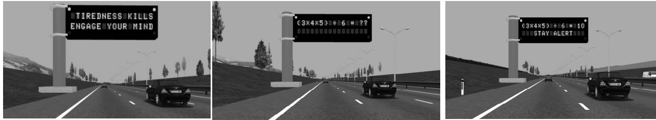
Figure 4. Variable message signs
