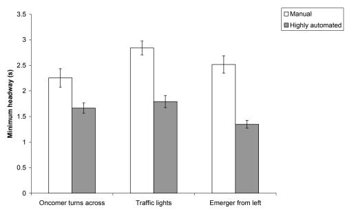
Figure 3. Drivers' minimum headway to the lead car during the manual and automated driving events
