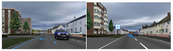
Figure 2. The road markings (left) and sign (right) used to denote the eLane
