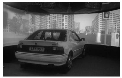
realistic sounds of engine and other noises via two speakers mounted close to each forward road wheel. Although the simulator is fixed-base, feedback is given by steering torques and speeds at the steering wheel. Data is collected at 30Hz and includes information of the behaviour of the driver (i.e. driver controls), that of the car (position, speed, accelerations etc.) and other autonomous vehicles in the scene (e.g.
