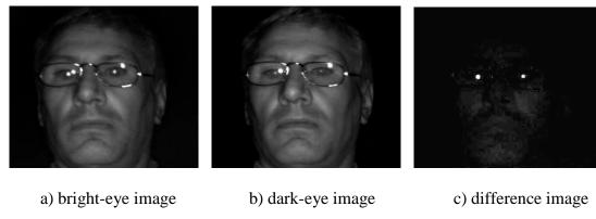
**Figure 1:** The three images used by the Copilot are shown above. The bright-eye image (a) and the dark-eye image (b) are essentially identical except for the glowing pupils in the bright eye image. The difference-image (c) eliminates all image features except for the bright pupils.
