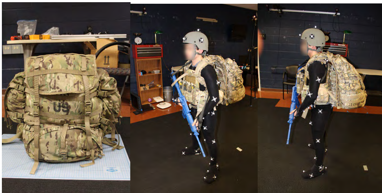
Figure 4. Participant with “sustainment load” configuration during motion capture sessions for select CSTs.
