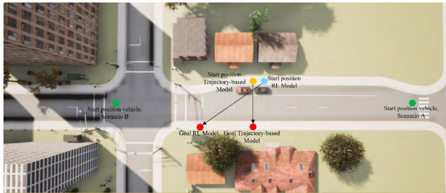
Figure 1 - A representation of the road. The blue mark indicates the initial position of the RL model and the orange mark of the trajectory-based model. The red is the destination of the pedestrian. The green mark is the start position of the vehicle. The road has 2 driving lanes and a parking lane with widths of 3.5 m. The arrows indicate the direction of movement of the pedestrian. The OpenDRIVE format was used to define the road network.
