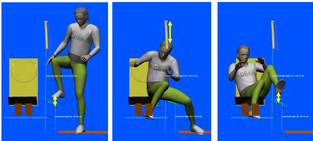
Figure 6 Collision avoidance of during car ingress (r. foot to sill, head to roof, l. foot to sill) (left to right)
