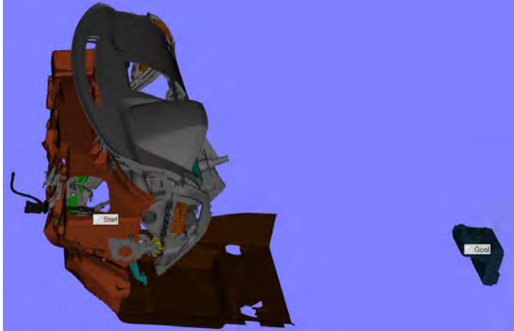
Figure 2. TC CEM Box: The CEM (central electronic module) box on the right side of the figure is the rigid body, whereas the parts of the dashboard on the left is considered to obstacles. Labels Start and Goal mark the rigid body's positions when it is assembled and disassembled, respectively.
