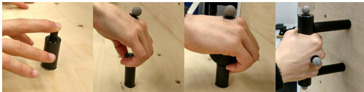
Figure 1. Grasping handles from left to right: One-finger contact, three-finger contact, ball, cylinder.
