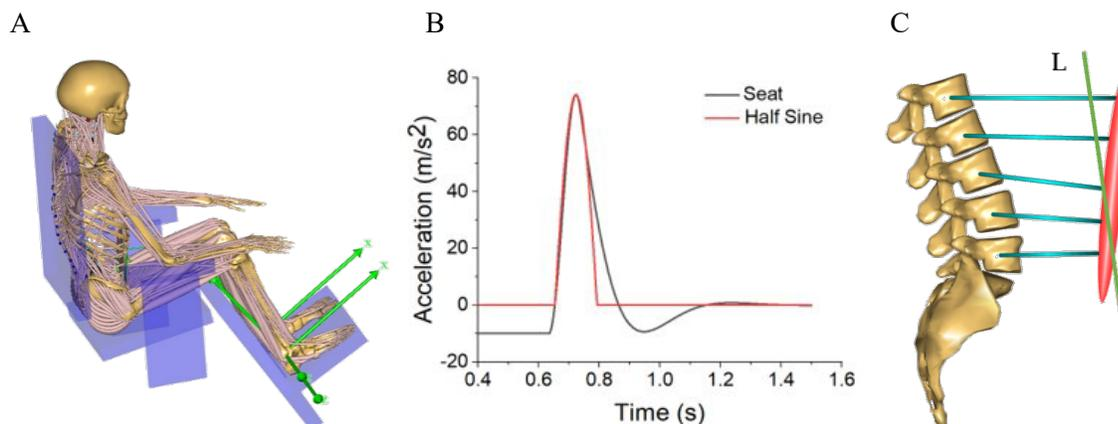
Figure 1. (A) A 3-D view of a seated human model in AnyBody software. (B) Half-sine pulse for simulation and the shock pulse on the seat surface. (C) Lumbar region structure with vertebra and transversus muscle.
