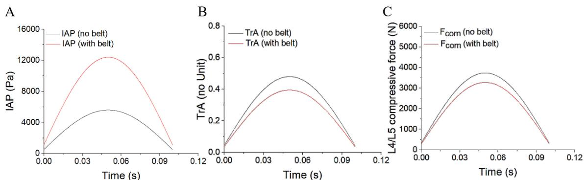
Figure 2. Belt effects on seated human model. (A) IAP value comparison. (B) Transversus muscle activity comparison. (C) Comparison of compressive force at L4/L5 joint.
