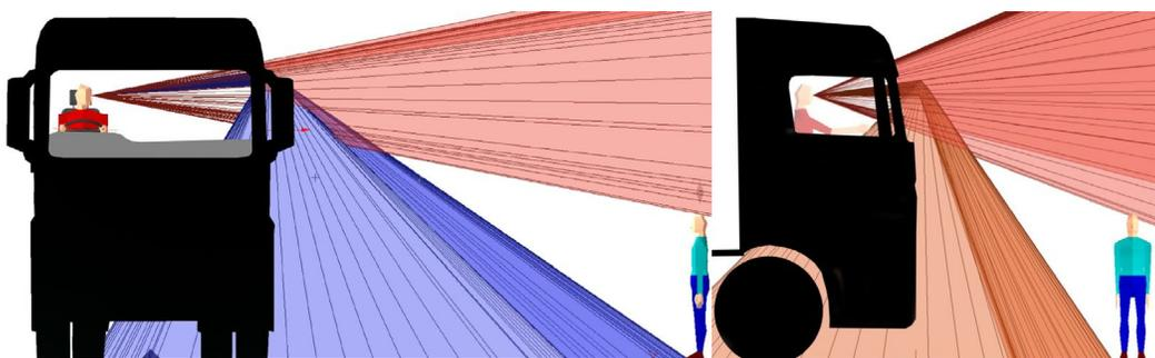
Figure 5. A situation in which the VRU simulation cannot be seen by the driver in either direct vision though windows or indirect vision through mirrors
