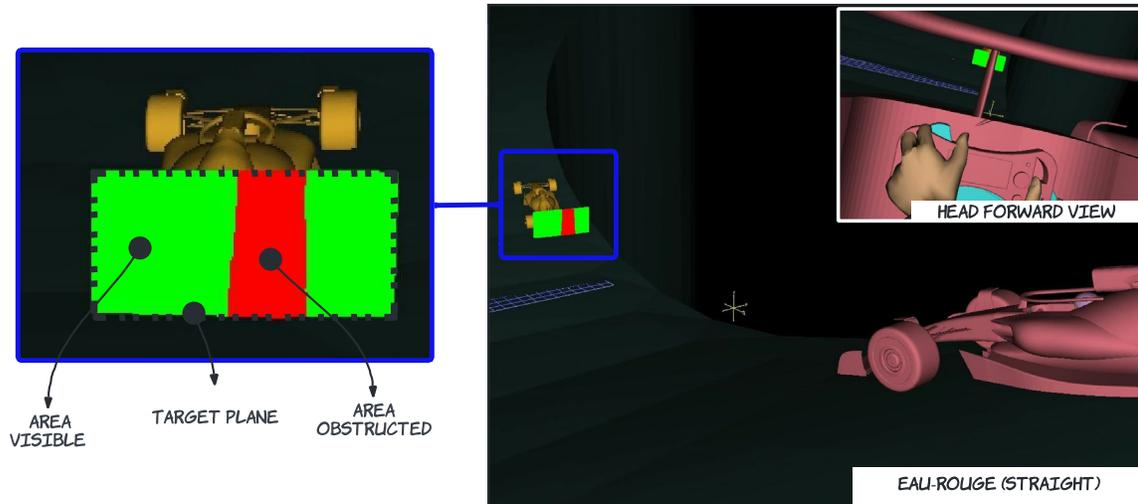
**Figure 6.** The image illustrates the *coverage zone* analysis performed in the 2022 F1 model with the thin-bar halo design. The area of the target plane (represented with dash lines) shaded in green represents the rays blocked by the vertical bar.
