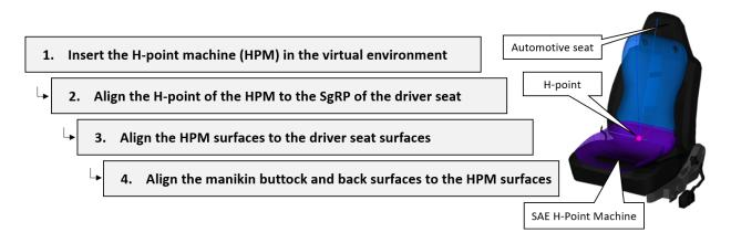
Figure 2. Body Shape Alignment approach.
