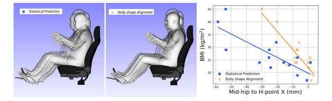
Figure 4. Initial seated driving posture: Statistical Prediction (left) and Body Shape Alignment (right).
