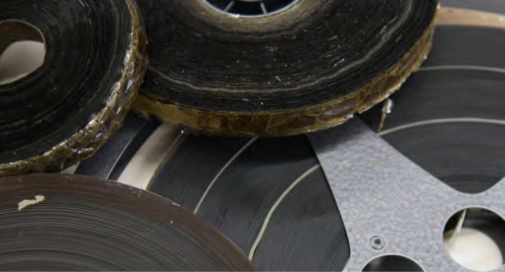
This image demonstrates the damage that can occur when reels are stored away for decades.
