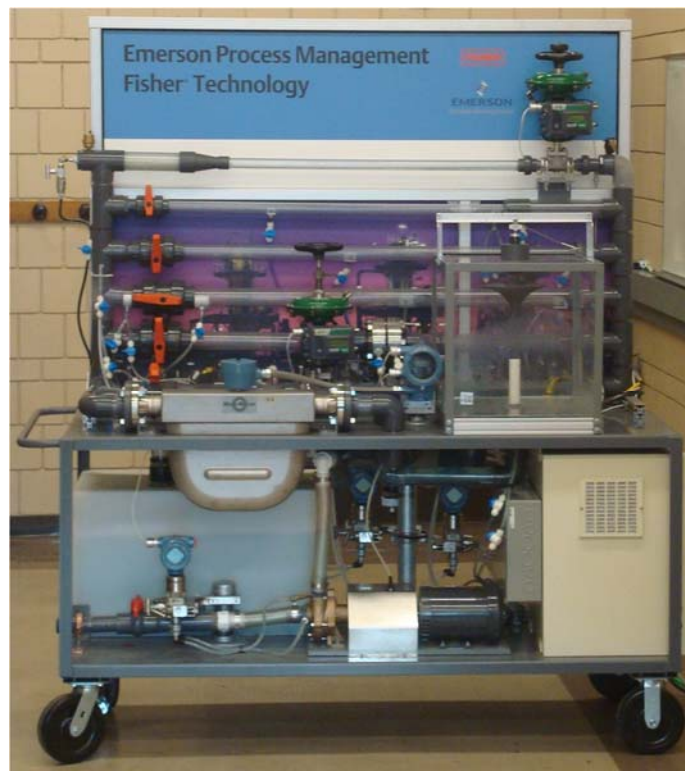
Figure 1. The experimental bench used for the fluids laboratory exercises. The bench was developed by Emerson-Fisher Controls several years ago for the fluids course.
