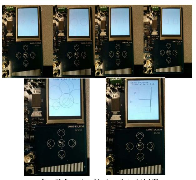
Figure 12 Four options of drawing on the touchable LCD (a) Two circles sample draw (b) Two squares sample draw (c) Draw circles (d) Draw squares
