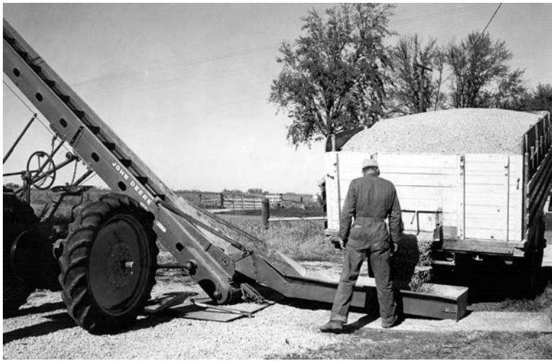
Grain elevators eased the arduous task of shoveling grain by hand. Unfortunately, farmers were sometimes caught in whirling PTO shafts or other rapidly moving parts of such devices. Photo from A. M. "Pete" Wettach Collection, State Historical Society of Iowa, Iowa City.
