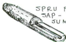
TRUNNELED SHOULDERED HICKORY PEGS CUT 8 SIDED HELD BETTER WHEN DRIVEN IN ROUND HOLE
