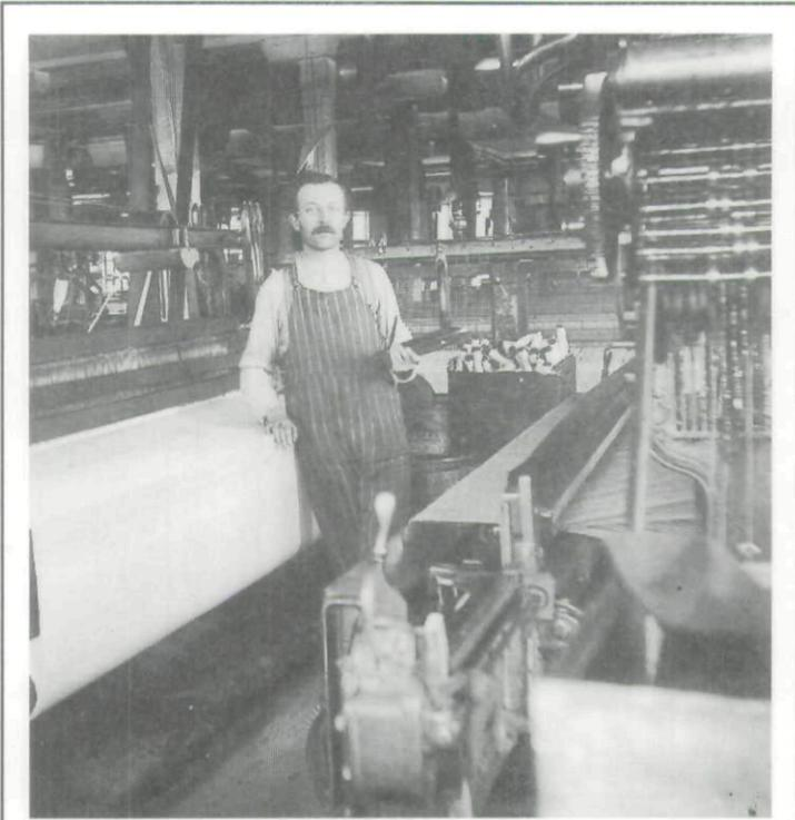
*Klaus Koenig, one of the outside workers hired by the Amana Society, is seen here in a rare interior view of one of the woolen mills, circa 1895, holding a shuttle and tending two belt-driven looms weaving flannel. Photo from SHSI, Iowa City.*
