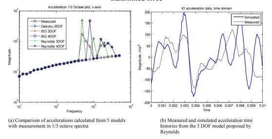
Fig. 2 Comparison of measured and semi-analytically estimated x-direction accelerations of an angle grinder.
