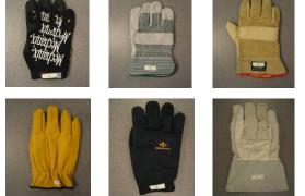
Fig. 1. The six gloves used in the study: (1) Mechanix Wear automotive (2) leather/cotton construction (3) Decade gel padded, antivibration (4) Impacto leather, air pocket, antivibration (5) Impacto mesh, air pocket, antivibration (6) ErgoAir pump, air pocket, antivibration
