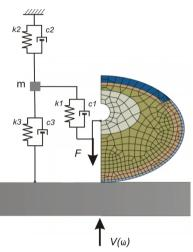
Figure 1: Hybrid model of a fingertip.
