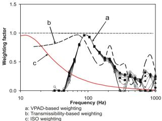
**Figure 3**: Comparison of the frequency weighting derived using VPAD with ISO-weighting and the weighting derived using the finger surface vibration transmissibility. The VPAD-based weightings were calculated using data at different locations within the soft tissues and shown in different symbols.
