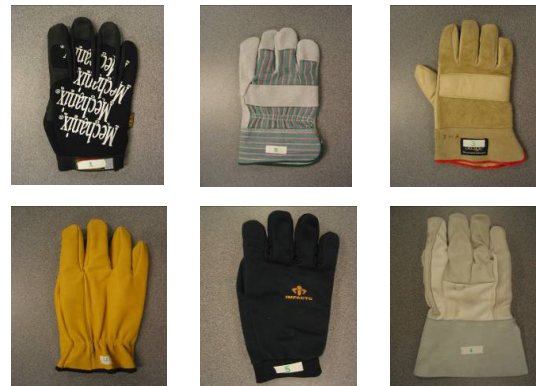
Fig. 1. The six gloves used in the study: (1) Mechanix Wear automotive (2) leather/cotton construction (3) Decade gel padded, anti-vibration (4) Impacto leather, air pocket, anti-vibration (5) Impacto mesh, air pocket, anti-vibration (6) ErgoAir pump, air pocket, anti-vibration
