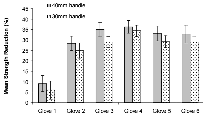
Figure 3. Mean grip strength percent reduction for the six gloves used in testing. (Y-error bars indicate the 95% confidence intervals for each mean).
